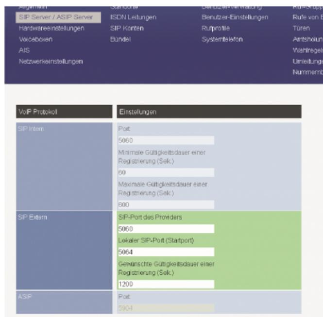
The screenshot shows the configuration interface for the ES-System. The 'SIP Server / ASIP Server' menu item is selected. The 'SIP Extern' settings are visible, including 'SIP-Port des Providers' (5060), 'Lokaler SIP-Port (Startport)' (5064), and 'Gewünschte Gültigkeitsdauer einer Registrierung (Sek.)' (1200). The 'ASIP' settings are also visible, including 'Port' (5904).
